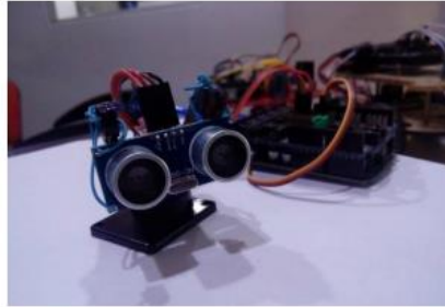
Figura. 2. Sensor HC-SR04, (VARGAS-Manuel, 2015).
